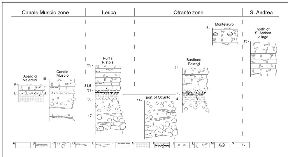
**Fig. 4** - Geological sections of the investigated areas. A - pre Pliocene; B - paleosol; C - Chaotic assemblage; D - undulated calcarenite beds; E - limestone and calcarenite lens; F - Marlstones; G - Glaucinitic siltstones; H - Phosphatized calcirudite; I - squashed marly inclusions; L - bioturbated calcarenites and limestones; M - *Arctica islandica* shells; N - meters from section base.
