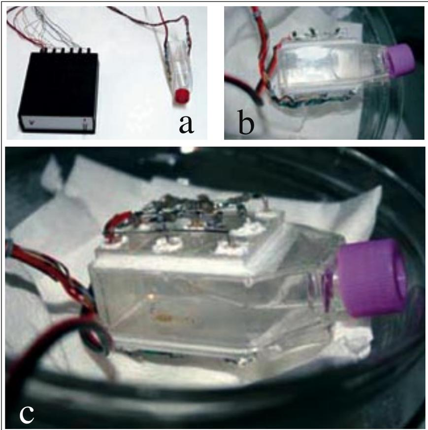
Fig. 1 - Pictures show the cell of recording and the connection to the electric circuit (a); cell view of side and position of the sensors (b). Cell and mysidacean in recording (c).
