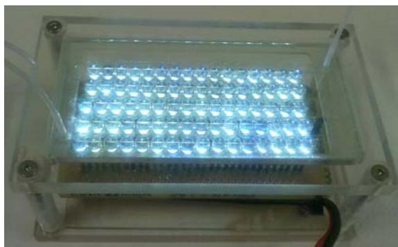
**Figure 1 - Photochemical microreactor with white LED illumination**
