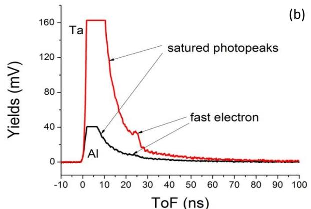
Fig. 2 Comparison between the spectra obtained irradiating Al and Ta targets (a). Detailed analysis of the two photopeaks which show and overlapping structure due to the presence of fast electrons (b).
