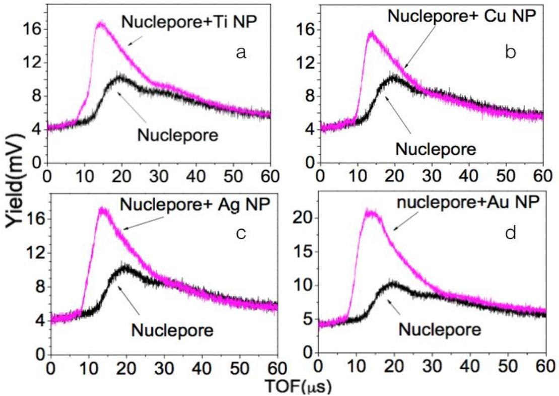
Fig. 4: Time of Flight spectra of nuclepore targets containing nanoparticles
