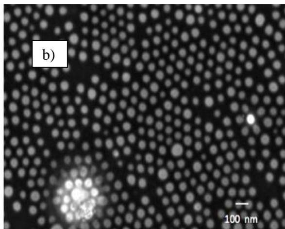
Fig. 2: Au NP Absorbance vs. wavelength (a) and TEM image of the Au produced nanoparticles (b)
