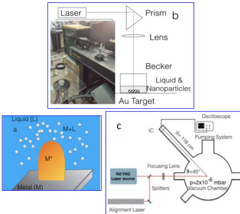
Fig. 1: Production of metal nanoparticles by laser ablation in a liquid (a), experimental apparatus for laser ablation (b) and set-up for the measurements of particles time of flight (c).
