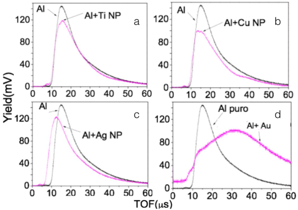
Fig. 3: Time of Flight spectra of Al targets with nanoparticles
