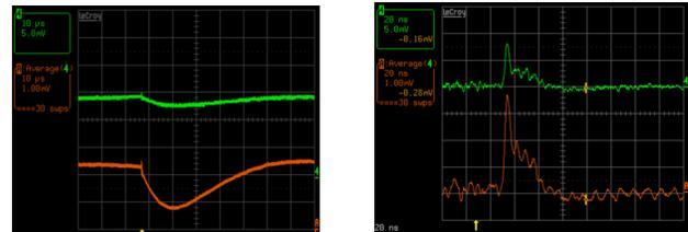
Fig. 8. Left: slow (10  $\mu$ sec/div; 5 mV/div) OGE; Right: fast (20 nsec/div; 5 mV/div) OGE.
