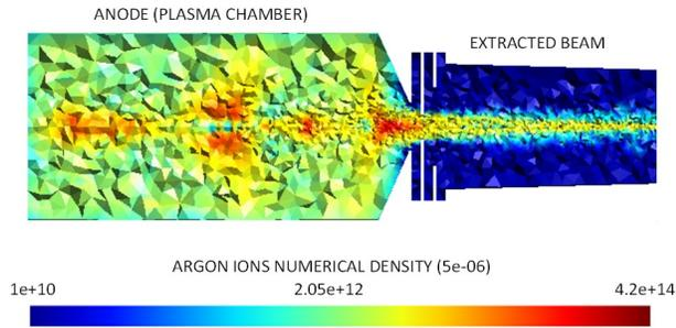
Fig. 6. Simulation of the SPIS extracted ion beam.
