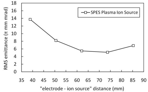
**Fig. 5b.** Measured RMS emittance for the SPES Plasma Ion Source.
