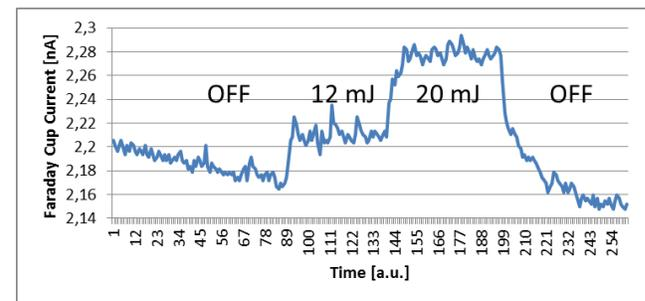
Fig. 11. Faraday cup current signal of ion collected under laser action in (up) proportional to several repetition rate value, (down) proportional to several energy pulse value.
