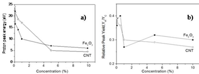
**Fig. 8:** The proton peak energy as a function of the doping concentration, for the forward detection configuration (a) and the relative peak yield between protons and carbon ions,  $Y_H/Y_C$ , as a function of the doping concentration (b).
