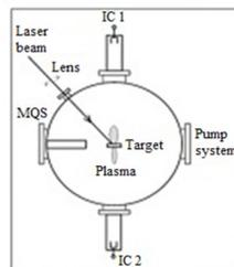
Fig. 1: A scheme of the experimental setup.
