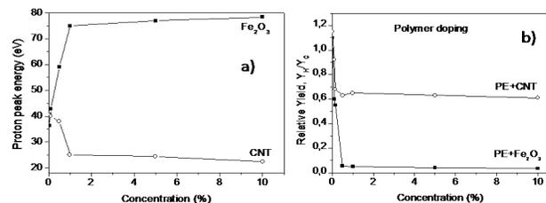
Fig. 6: The proton peak energy as a function of the doping concentration, for the backward detection configuration (a) and the relative peak yield between protons and carbon ions,  $Y_H/Y_C$ , as a function of the doping concentration (b).
