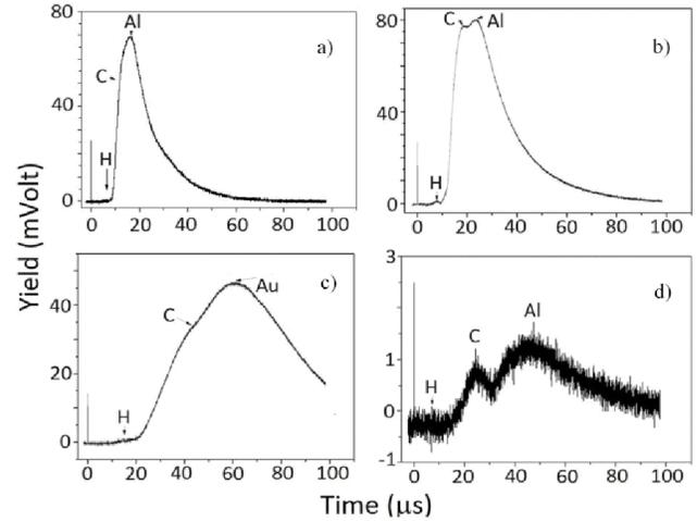
**Fig. 3:** Four typical IC2-TOF spectra obtained by irradiating from the polymer side the 2  $\mu\text{m}$  mylar film covered by 0.1  $\mu\text{m}$  Al (a), the 3.5  $\mu\text{m}$  mylar film covered by 0.1  $\mu\text{m}$  Al (b), the 100  $\mu\text{m}$  mylar film covered by 500  $\text{\AA}$  Au (c), and by irradiating from the metal side, the 0.1  $\mu\text{m}$  Al thin film covering 2  $\mu\text{m}$  mylar film (d) and detecting the ion emission in forward direction.
