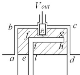
Fig. 4. Cross section of the modified divisor electrode.
