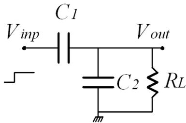
Fig. 2. Schematic diagram of a capacitive voltage divisor:  $C_1$  is the capacitance of divisor electrode and external conductor,  $C_2$  is the capacitance of the internal conductor and the divisor electrode.
