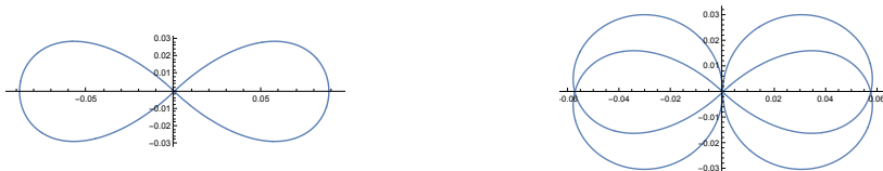
Fig. 10 : \gamma_2(t) = \left( \frac{\cos^3 t \sin^3 t}{\sqrt{2}}, \frac{\cos^3 t \cos 2t \sin^3 t}{\sqrt{2}} \right) . Fig. 11 : The 0-pedaloid of \gamma_2 .
