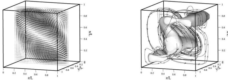
Figure 1. Laminar natural convection flow in a cubical cavity at Rayleigh number  $3 \cdot 10^4$  and Prandtl number 0.7. Left: Vector field in the plane  $y/L=0.5$ . Right: Three-dimensional view of the isosurface  $B/B_{max} = 0.75$  and some particle paths.
