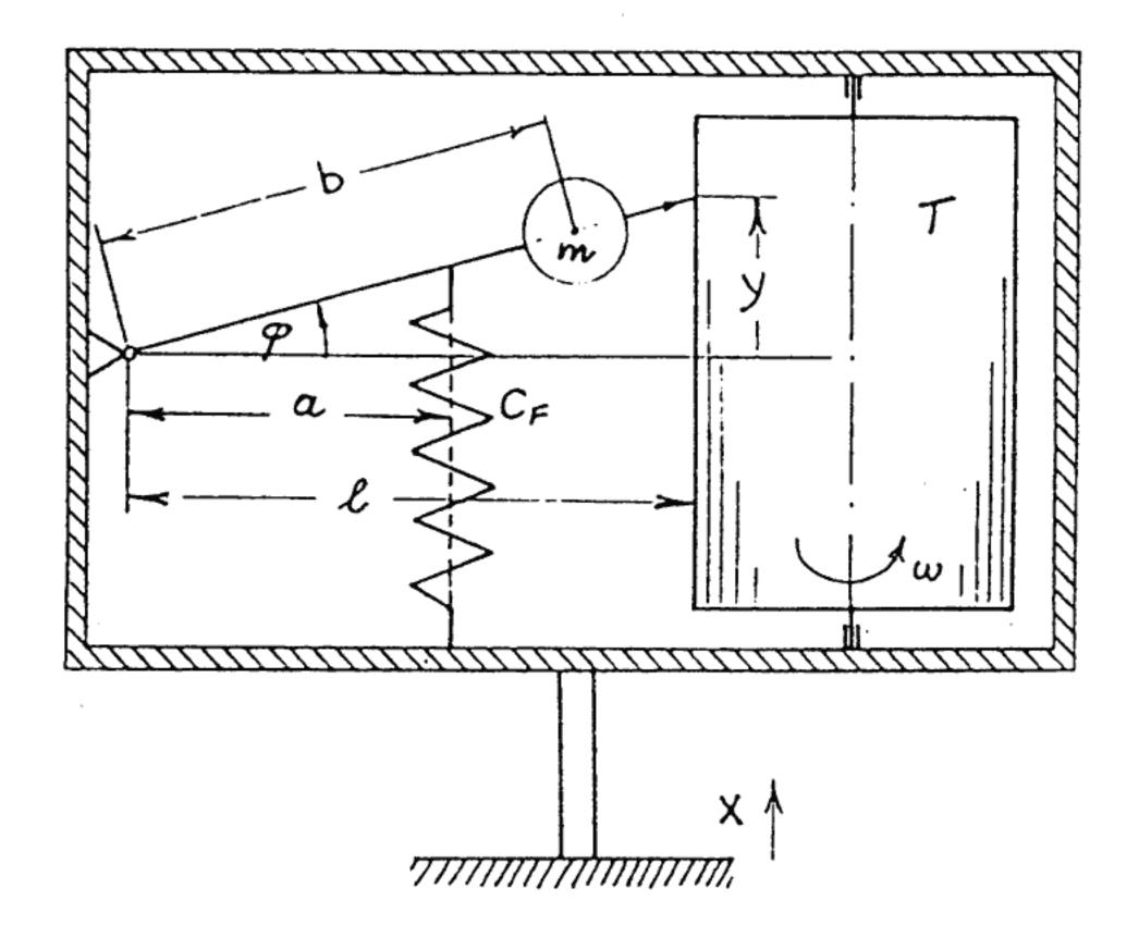
Vibrations x of the earth surface move the box. By inertia the mass m tries not to move, and so we get a movement of the mass relative to the box that is written onto the cylinder T which turns with a constant speed  $\omega$ .
