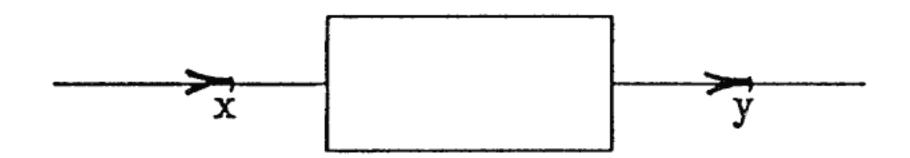
which transforms a linear space of input signals  $x : \mathbb{R} \to \mathbb{R}$  into output signals  $y : \mathbb{R} \to \mathbb{R}$ , y = A(x), belonging to another linear space. Linearity of the transfer system means linearity of the mapping A.
