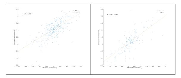
Figure 1: Plot of computed accelerations  $(\hat{A}_t)$  in  $m.s^{-2}$  versus measured accelerations  $(\hat{A}_t)$   $m.s^{-2}$  for runner 2, intensity Medium (Left) and for runner 5, intensity Hard (Right).
