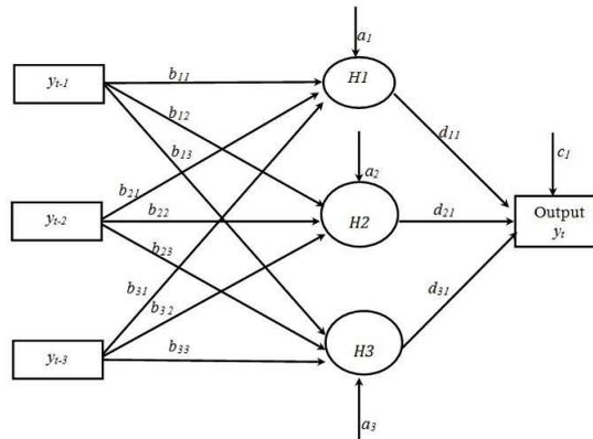
Figure 1: Diagrammatic representation of ANN ( $i, j, k = 3$ ) where  $i$  is the number of inputs,  $j$  number of neurons in the hidden layer and  $k$  lag period.
