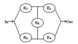
Figure 1. Diagram of five unit bridge network.
