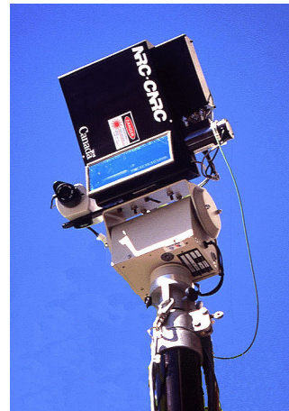
Figure 1. (a) The High Resolution Color Laser Scanner imaging a figurine. (b) The Biris 3D Laser Camera is a compact and robust monochrome camera for field recording applications. (c) The Large Volume “Big Scan” Laser Scanner is used for scanning large sites and structures.
