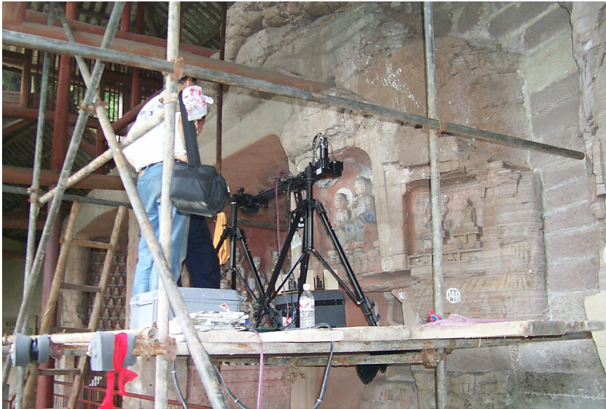
Figure 4: (a) The Large Volume or Big Scan Scanner set up to scan the entrance to the the Arcosolia Room of the Tomb of St. James in Israel. The camera is shown mounted on a tripod with the computer controller on the right. (b) The Biris camera set up on a linear translation stage to scan Niche #147 at the Buddhist rock carving site at Dazu in China.
