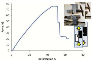
Fig. 4 - Typical force/deformation curve of a joint UH-UH/B.M. In the frames: magnification of a joint during a shear test (above) and force directions applied to the welded sheets (below).
